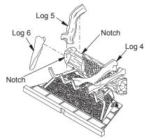
Figure 27 - Installing Logs 5 and 6
